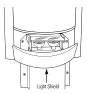
**WARNING** — The light shield must be replaced or the heat from the bulb could damage the refrigerator.
